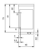
E: Electric power D: Drain for water
