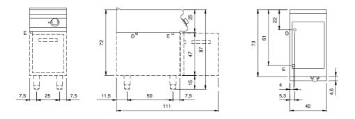
E: Electric power D: Drain for water
