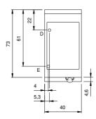
E: Electric power D: Drain for water
