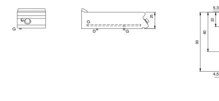
G: Gas connection 1/2" D: Drain for water
