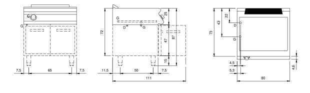
G: Gas connection 1/2" D: Drain for water
