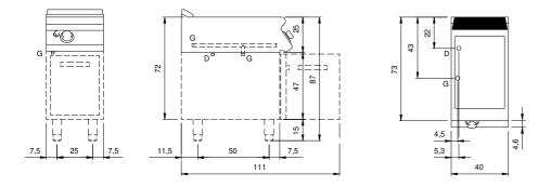
G: Gas connection 1/2" D: Drain for water
