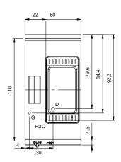
G: Gas connection 1/2" E: Electric power D: Drain for water
