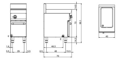
E: Electric power D: Drain for water H2O: Water inflow 3/4"
