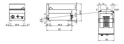
E: Electric power D: Drain for water H2O: Water inflow 3/4"
